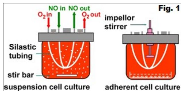
To combat these problems, researchers at MIT developed a novel, controllable, membrane-diffusion gas delivery system for cell culture studies, shown in Fig. 1<sup>3</sup>. Designed to be inexpensive and simple to fabricate, the system is essentially a modified chemostat. It avoids gas-phase NO chemistry and is capable of producing steady-state concentrations of O<sub>2</sub> and NO that mimic those
